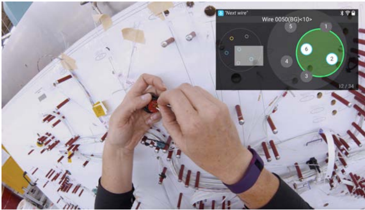
Boeing end-user point of view using Skylight on smart glasses.
