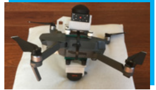
A DJI Mavic Pro drone outfitted for 360° video capture with 3D printed mounts and Kodak SP360 4K cameras Courtesy of Ben Kreimer for Making Waves
